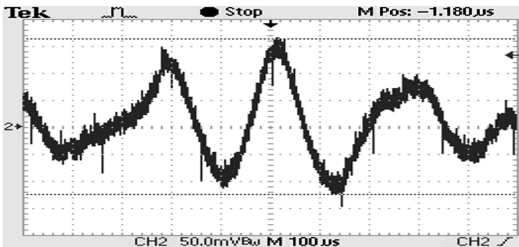
Figure 4.8: Ripple at the output of converter (without QEC) Y axis scale : 50 mV, X axis scale : 100  $\mu$ sec
