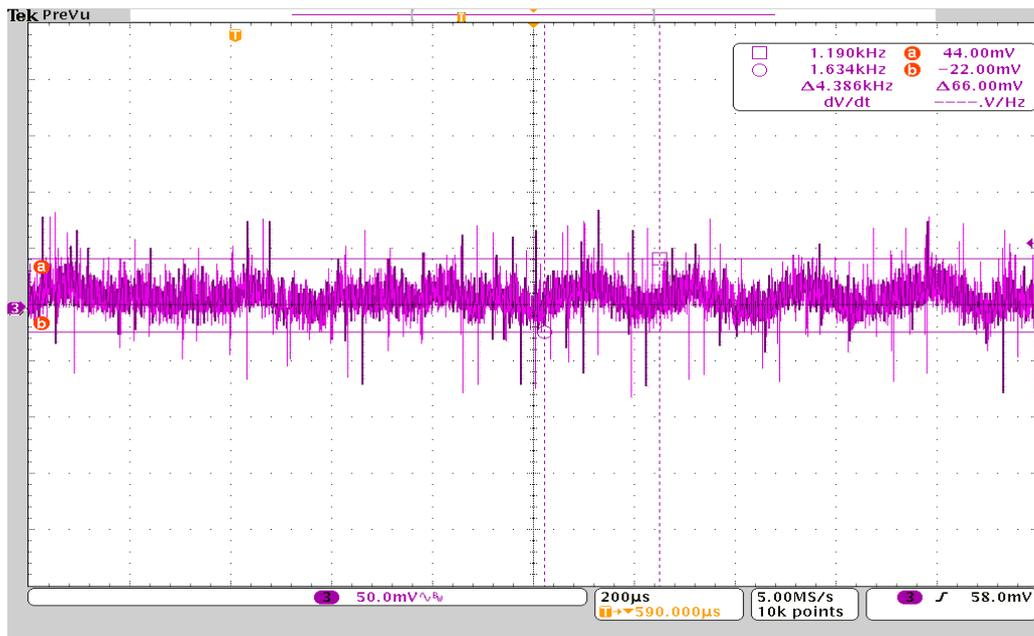
Figure 5.10b: Output of the converter with QEC. Input voltage of 18 V and load condition of 2A
