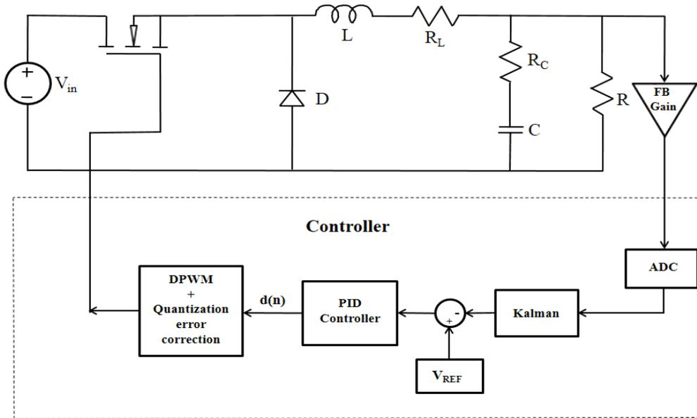
Figure 5.1a: Block diagram of the configuration of digitally controlled DC-DC converter combining reduced state Kalman filter and QEC
