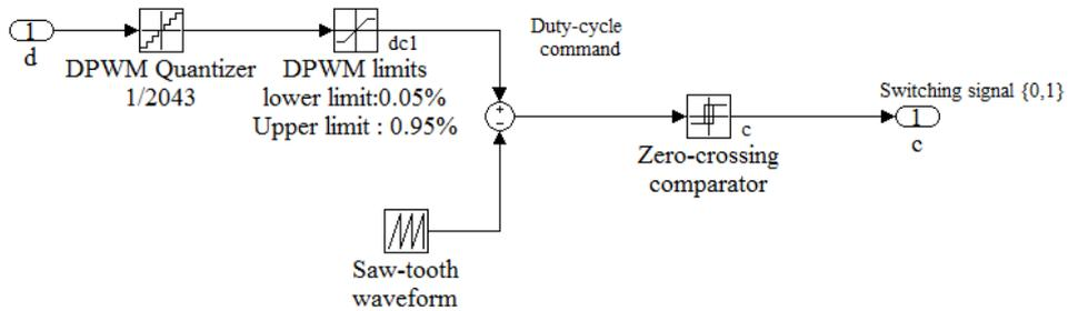
Figure 3.3b: Simulink model of the DPWM
