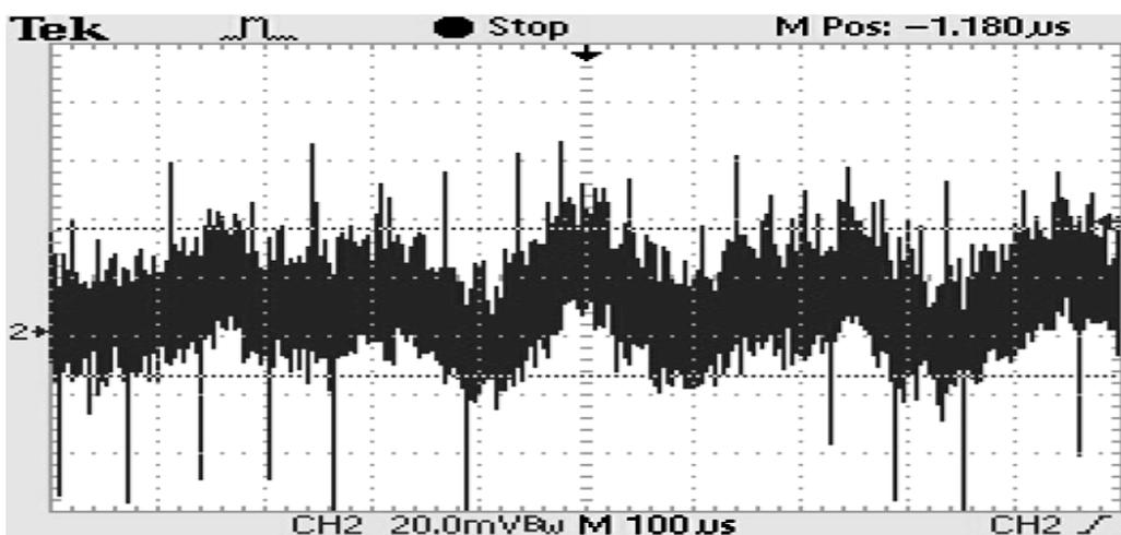
Figure 4.9: Ripple at the output of converter (with QEC) Y axis scale:20 mV, X axis scale:100  $\mu$ sec
