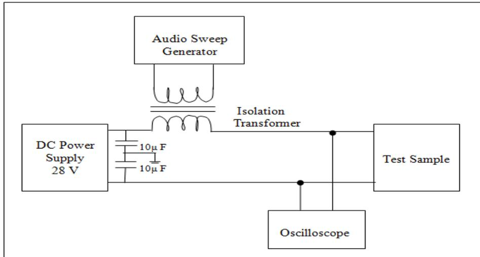
Figure 3.19: CS01 test of MIL STD 461C
