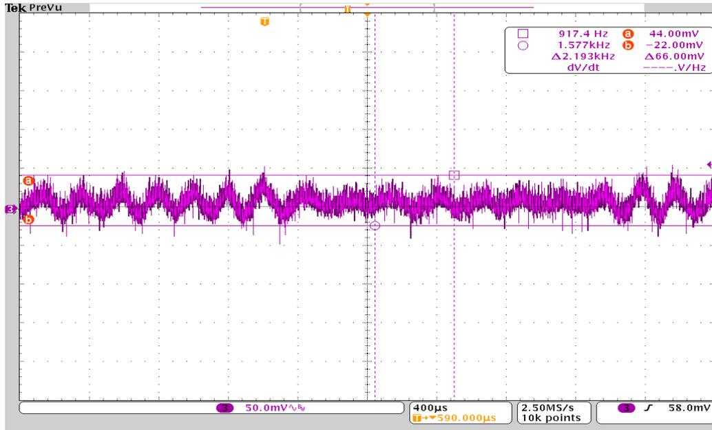
Figure 5.10a: Output of the converter with QEC. Input voltage of 18 V and load condition of 500 mA
