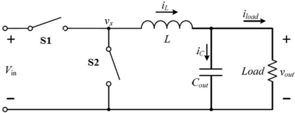
Figure 1.2: Configuration of buck converter [74]
