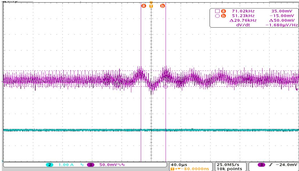
Figure 5.9c: Output of the converter with Kalman Filter (purple trace), Input voltage of 12 V and load condition of 2A. The load current is shown by blue trace.
