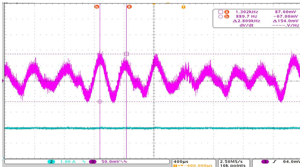
Figure 5.8b: Output of the converter with no error correction (pink trace), Input voltage of 18V and load condition of 2A. The load current is shown by blue trace
