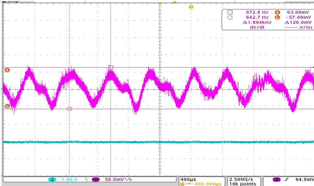
Figure 5.8c: Output of the converter with no error correction (pink trace), Input voltage of 12V and load condition of 2A. The load current is shown by blue trace.
