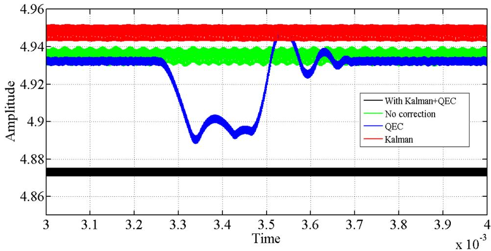
Figure 5.7: Output of converter, 8-bit ADC and 9-bit DPWM, Input voltage 18 V and load current of 2A
