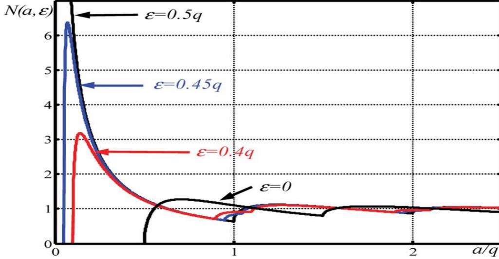
Figure A1.3: Describing function of a quantizer for several different values of the offset
