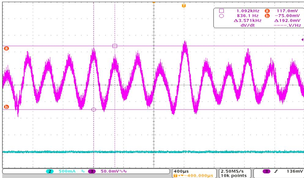
Figure 5.8a: Output of the converter with no error correction (pink trace), Input voltage of 18V and load condition of 500mA. The load current is shown by blue trace
