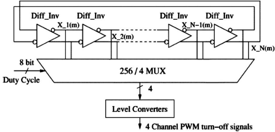
Figure 2.7: A ring oscillator MUX implementation of DPWM [1]
