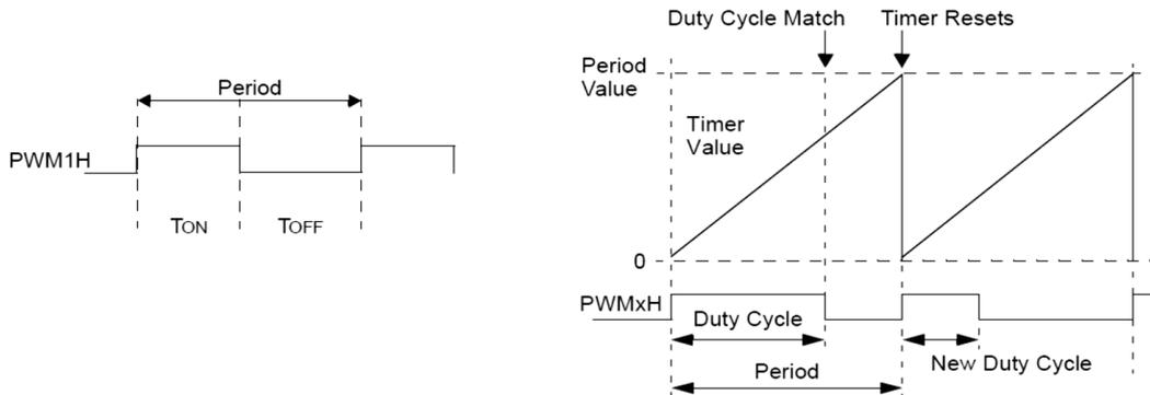
Figure 3.10: Standard edge aligned PWM
