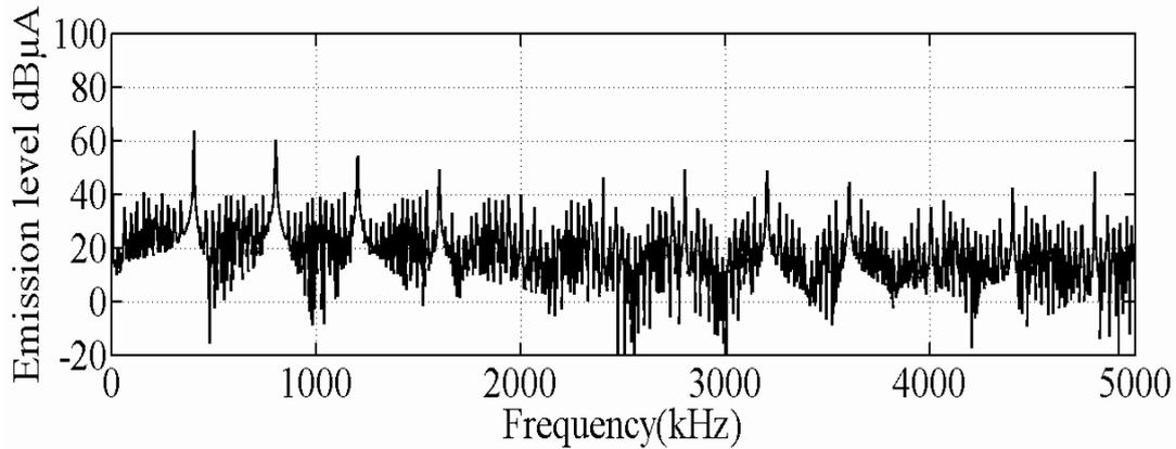
Figure 4.6: Simulation results showing emission level without QEC
