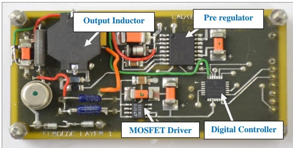
Figure 3.11: Prototype set up of the proposed scheme
