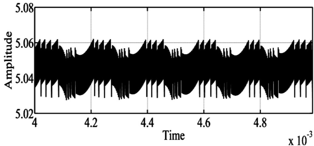
Figure 4.4: Simulation results showing the ripple at the output of the converter without QEC
