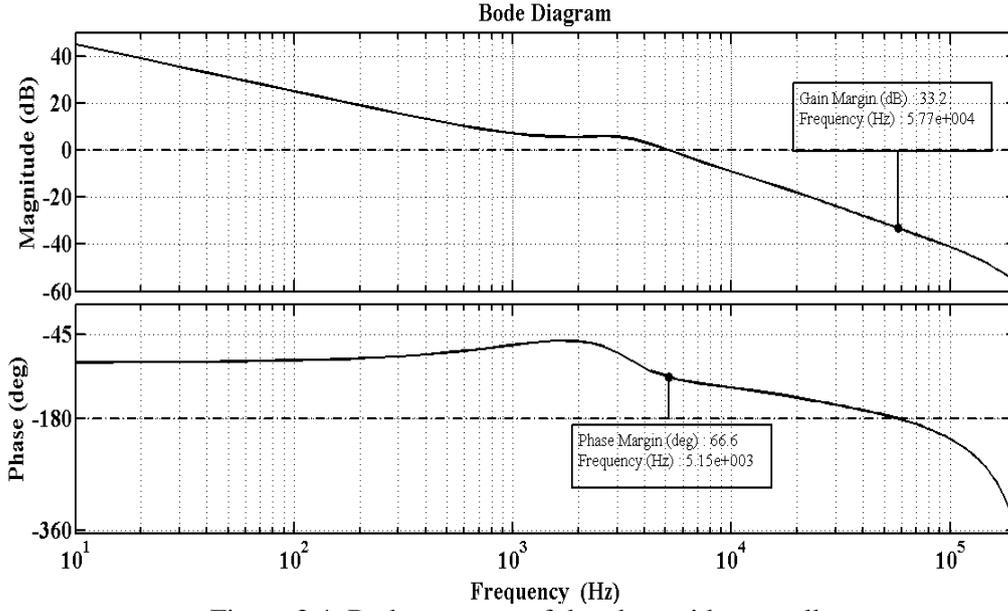
Figure 3.4: Bode response of the plant with controller
