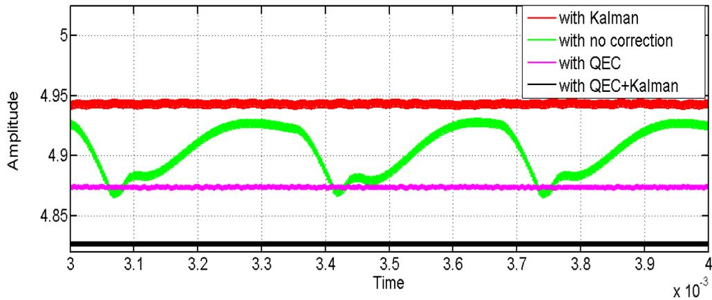
Figure 5.5: Output of converter, 6-bit ADC and 7-bit DPWM, Input voltage 12 V and load current of 2 A
