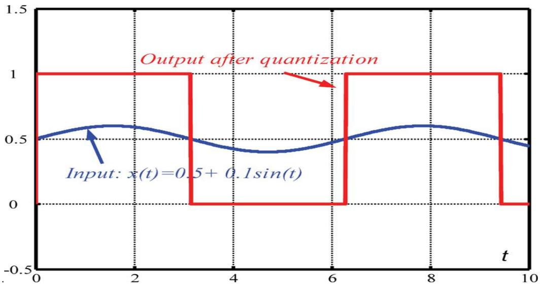
Figure A1.2: Small amplitude sinusoidal signal becomes square wave signal with much bigger amplitude when the DC offset  $\varepsilon$  of the input sinusoidal signal matches the transition point ( $0.5q$ ) between two quantization bins [4]
