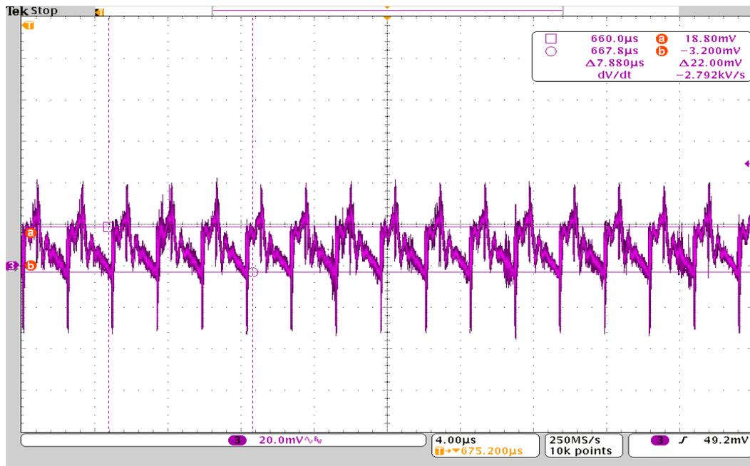
Figure 5.11: Output of the converter with Kalman filter and QEC
