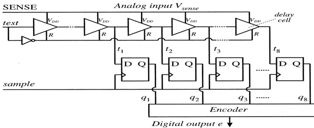
Figure 2.3: Basic delay line ADC [2]
