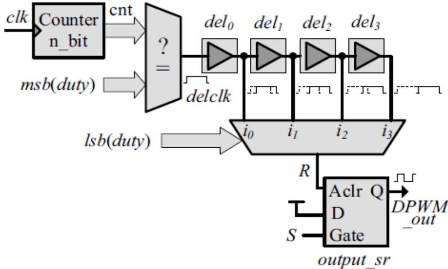
Figure 2.6: Hybrid DPWM with external clock [11]
