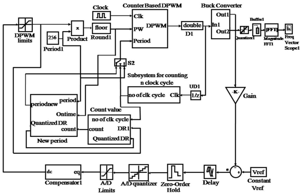
Figure 4.2: Simulink model of the digitally controlled DC-DC Converter with quantization error correction
