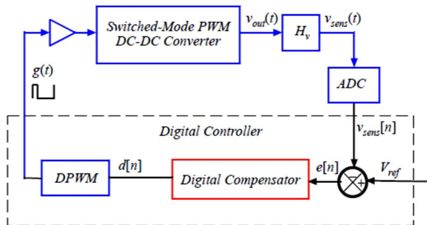
Figure 1.5: Block diagram of digitally controlled DC-DC converter
