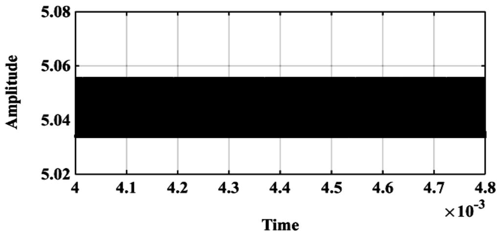
Figure 4.5: Simulation results showing the ripple at the output of the converter with QEC
