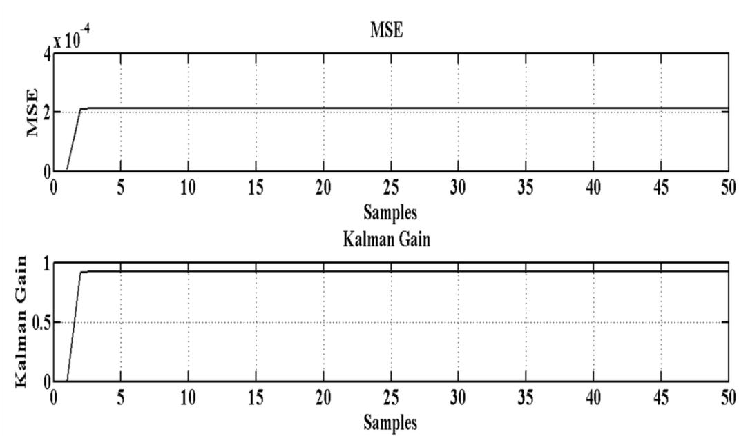
Figure 3.5: Mean square error and Kalman gain for 6-bit ADC and Vref: 1.6405 V
