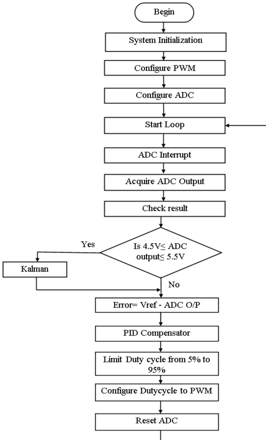
Figure 3.12: Flowchart of the controller implementation in dsPIC
