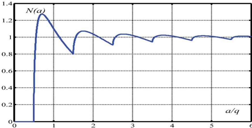
Figure A1.1: Describing function of a quantizer when the DC offset is  $\varepsilon = 0$ , i.e., the DC value of the input sinusoidal signal matches the midpoint of a quantization bin. [4]
