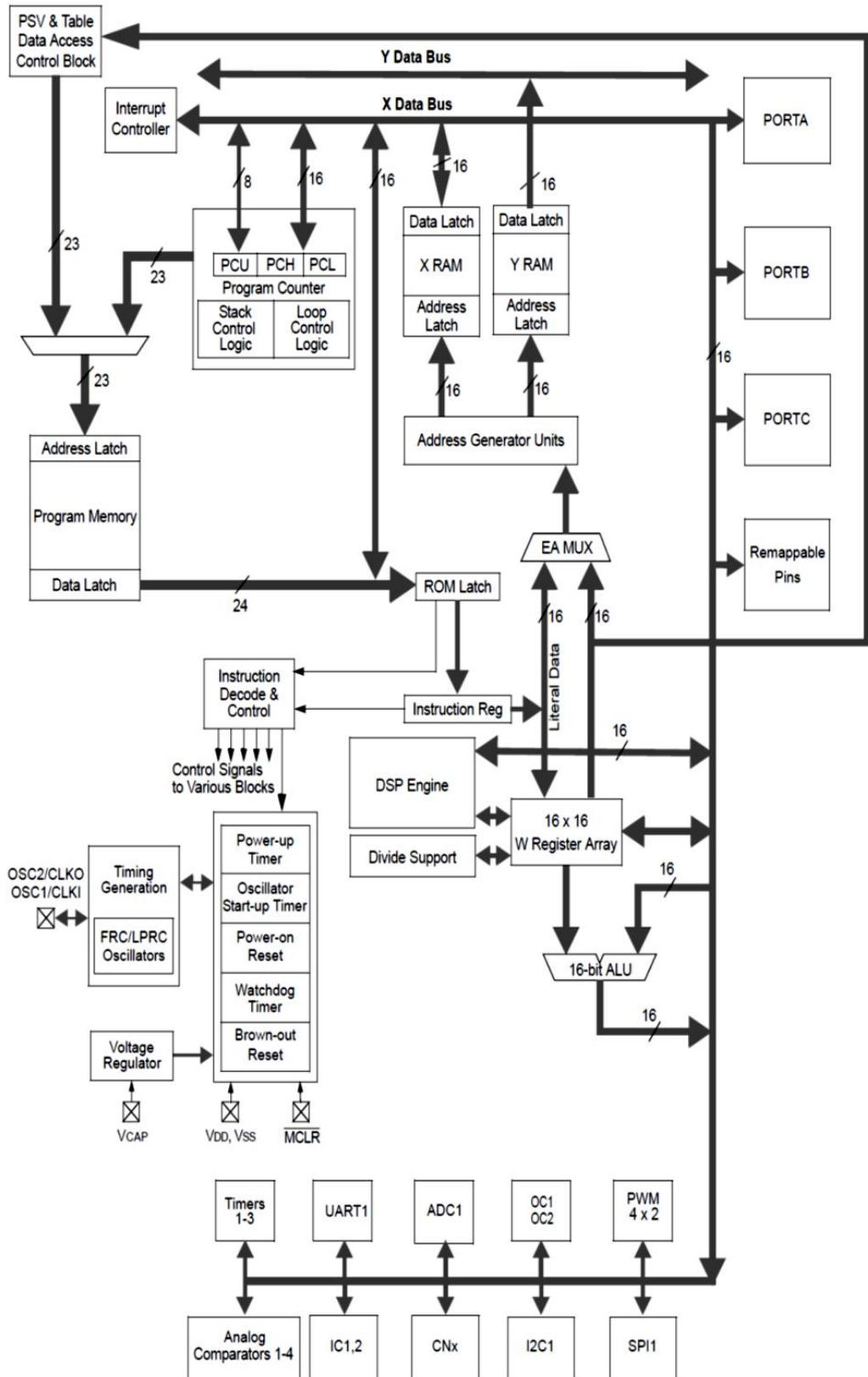
Figure 3.8: Block diagram of the core and the processor modules
