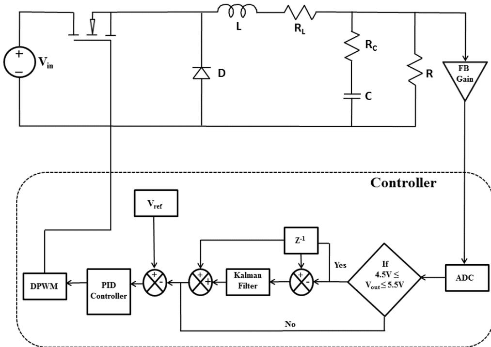
Figure 3.1: Block diagram representation of the proposed architecture
