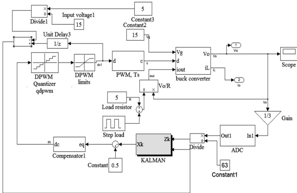
Figure 3.3a: Simulink model of the DC-DC converter with Kalman filter
