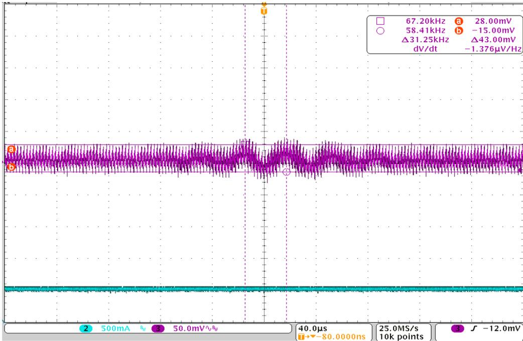
Figure 5.9a: Output of the converter with Kalman Filter (purple trace), Input voltage of 18 V and load condition of 500 mA. Load current is shown by blue trace.
