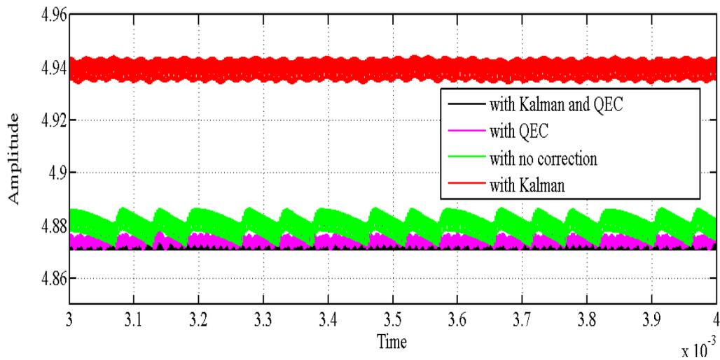
Figure 5.3: Output of converter, 6-bit ADC and 7-bit DPWM, Input voltage 18 V and load current of 2A
