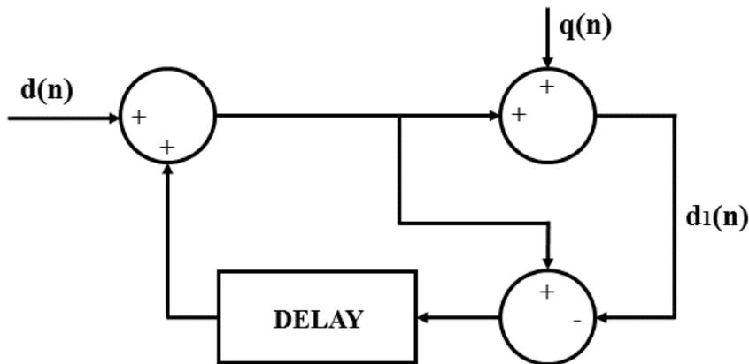
Figure A3.1: Sigma Delta Modulation Scheme
