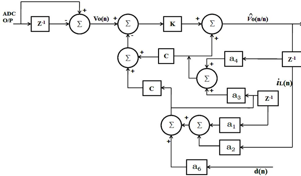
Figure 3.2: Block diagram of the scalar state scalar observation Kalman filter
