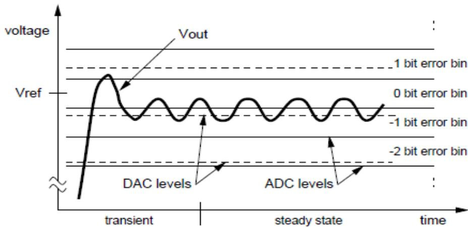
Figure 2.1: Qualitative behavior of output voltage ( $V_{\text{out}}$ ) for DPWM resolution less than ADC [3]
