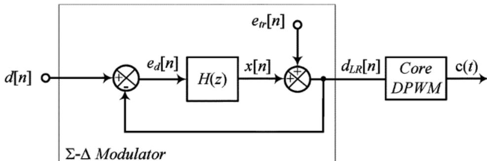
Figure 2.10: Multi bit digital sigma delta modulator [16]
