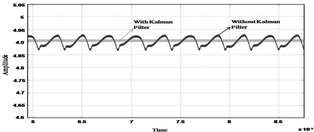
Figure 3.6: Output voltage response with and without Kalman (X axis:  $6.125 \times 10^{-3}$  to  $8.75 \times 10^{-3}$  sec, X axis scale:  $0.5 \times 10^{-3}$  sec, Y axis scale: 0.05 V)
