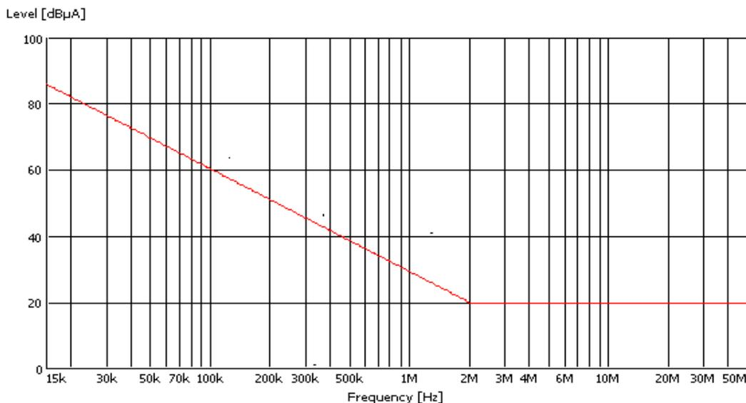
Figure A4.1: MIL-STD 461C Limit for conducted emission CE03 narrow band
