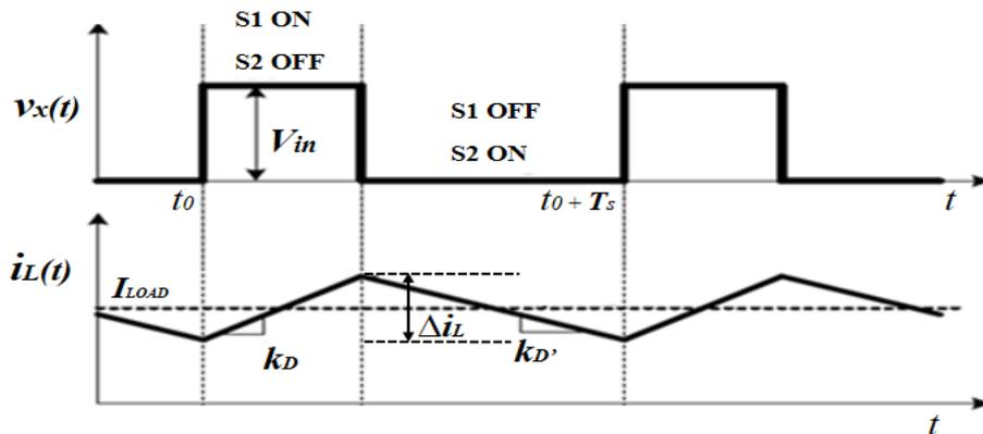
Figure 1.3: Steady State waveforms of buck converter in CCM [74]
