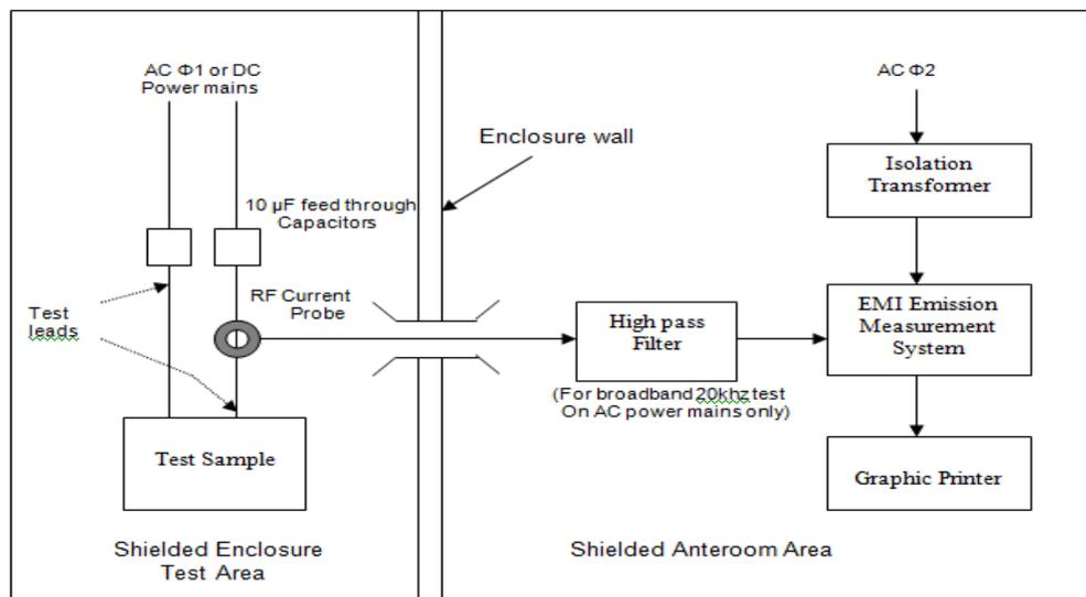
Figure A4.2: Test set up for CE03 power lead measurements
