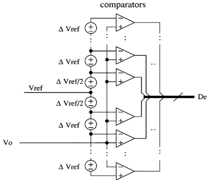
Figure 2.2: Flash window type ADC [1]
