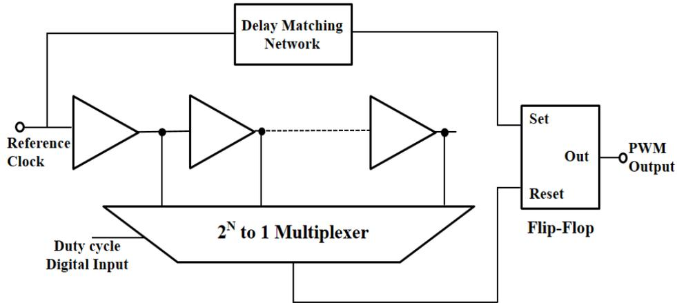
Figure 2.5: Delay line based DPWM [9]
