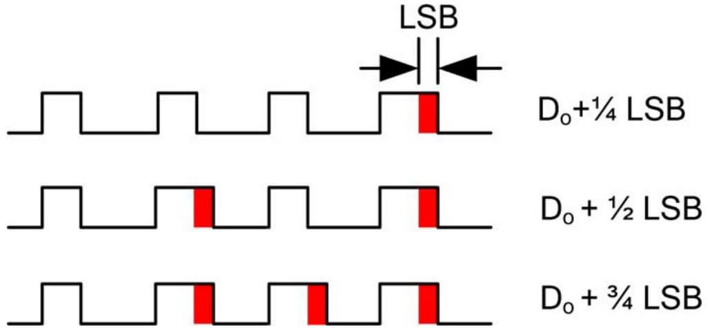
Figure 2.9: Scheme of digital dithering [3]
