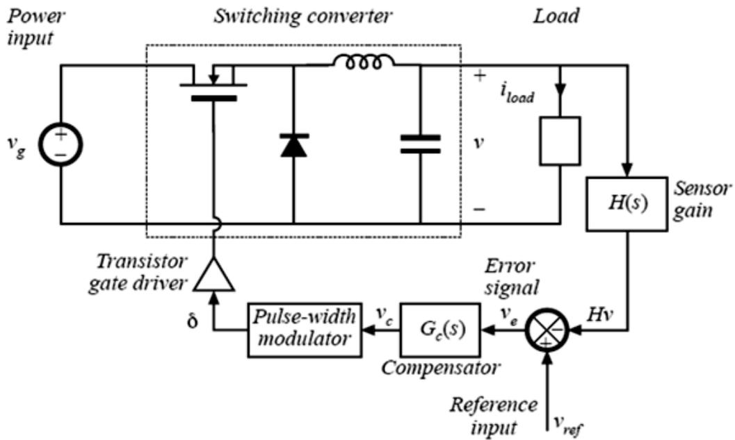
Figure 1.4: Block diagram of buck DC- DC converter using analog controller [75]
