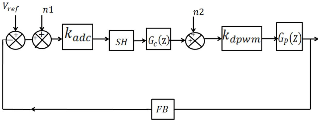
Figure A2.1: System model used for the calculation of process noise
