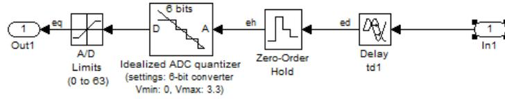
Figure 3.3c: Simulink model of the ADC
