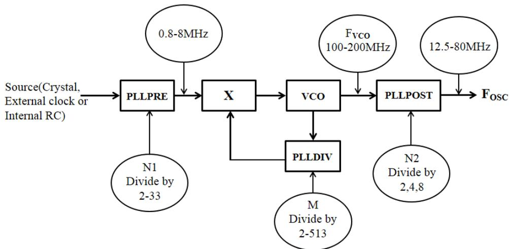
Figure 3.9: Oscillator portion of the dsPIC
