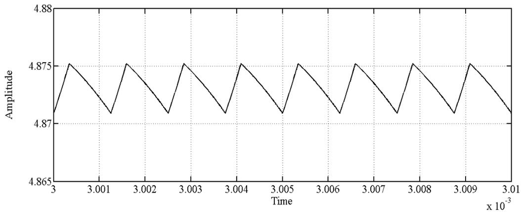
Figure 5.4: Output of converter, 6-bit ADC and 7-bit DPWM, Input voltage 18 V and load current of 2 A with Kalman & QEC (expanded view)
