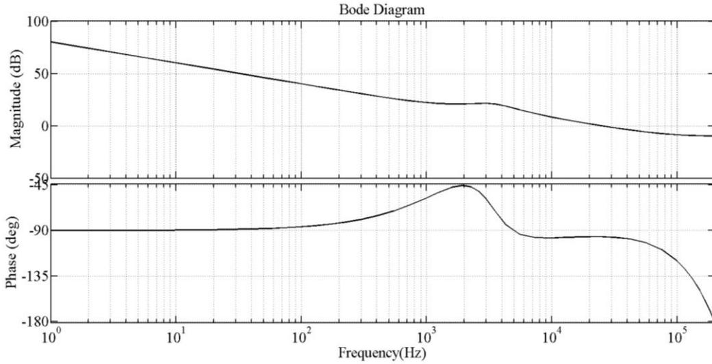
Figure 4.3: Open loop response of the converter (converter and compensator)
