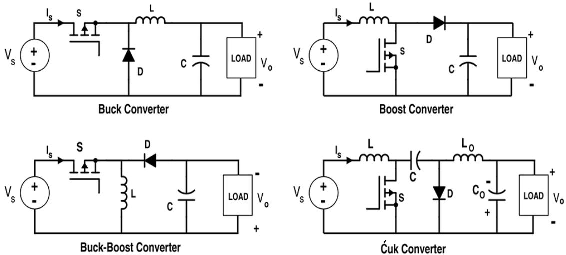
Figure 1.1: Basic non-isolated converter topologies
