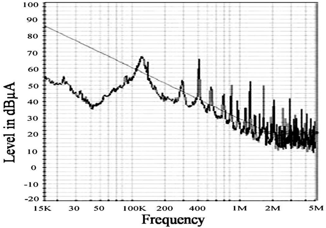
Figure 4.11: Conducted emission level without QEC (CE03 test of MIL STD 461C)
