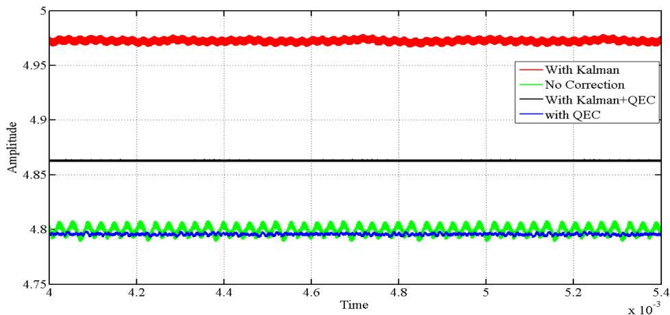
Figure 5.6: Output of converter, 5-bit ADC and 6-bit DPWM, Input voltage 12 V and load current of 500 mA
