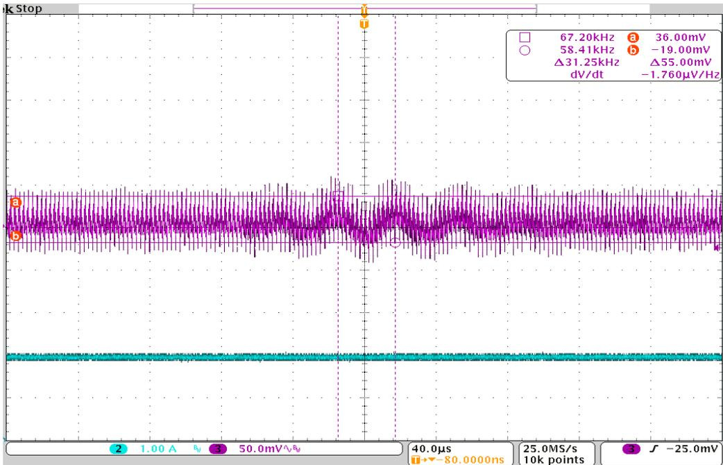
Figure 5.9b: Output of the converter with Kalman Filter (purple trace), Input voltage of 18 V and load condition of 2 A. The load current is shown by blue trace.
