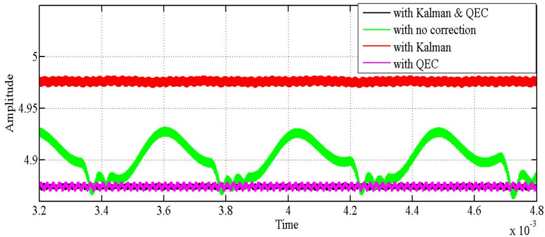
Figure 5.2: Output of converter, 6-bit ADC and 7-bit DPWM, Input voltage 18 V and load current of 500 mA.
